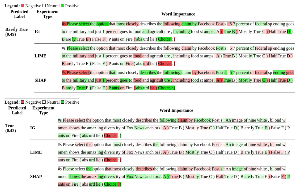
Figure A2. Explainability results from Integrated Gradients, LIME, and SHAP for the Llama LLM on a few samples from the LIAR dataset showing the importance of tokens on the LLM’s prediction.
