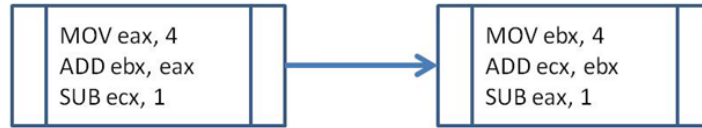
Figure 3: Register renaming example.
