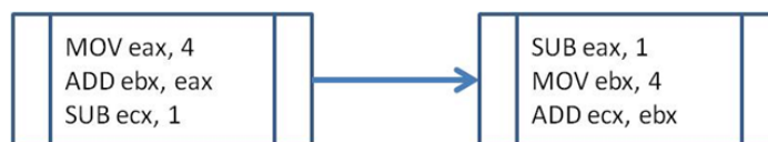
Figure 5: Instruction reordering and equivalent instructions substitution.
