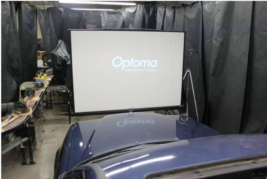
Figure 4. Black paper curtains used to darken experimental area can be seen surrounding the car.
