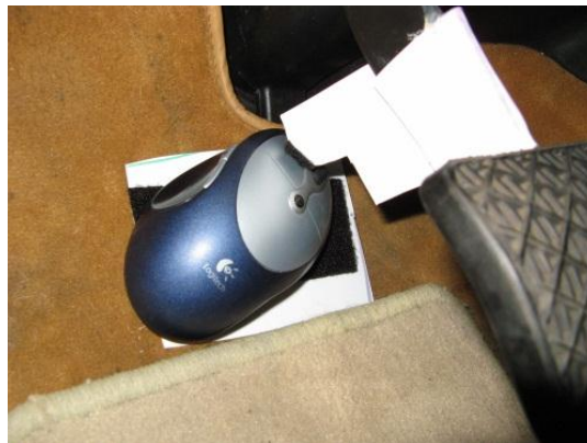
Figure 9. Wireless mouse placed under brake pedal, with actuator arm attached to pedal.
