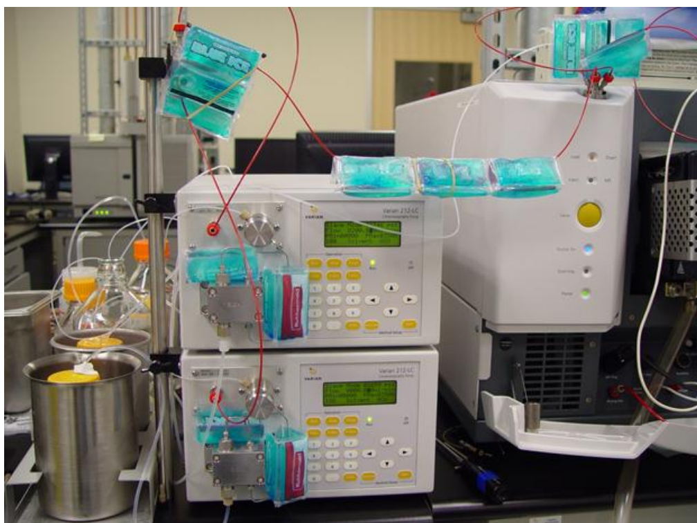
Fig. 7. HPLC lines and pumpheads wrapped in propylene glycol ice packs.
