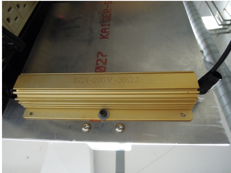
Figure 3.12: A 30\ \Omega 200\ \text{W} power resistor mounted onto aluminum plate, which is mounted onto the rolling cart. The resistor provides a dummy load to run the projector without the original lamp.
