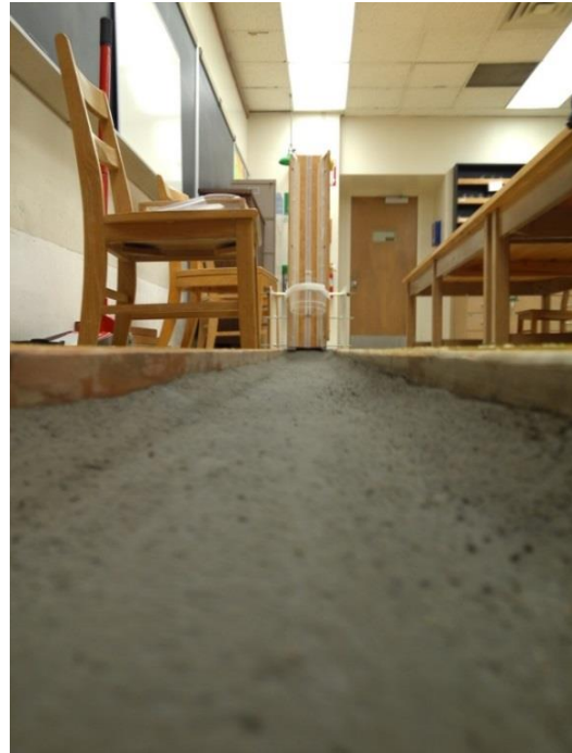
Figure 4. Picture of the dry ravel flume surface. The sides of the flume are slightly curved to prevent particle collision with the wooden sides of the flume. The clear acrylic sediment chamber can be seen in the background. The sediment chamber is strapped by Velcro so that the elevation can be adjusted.
