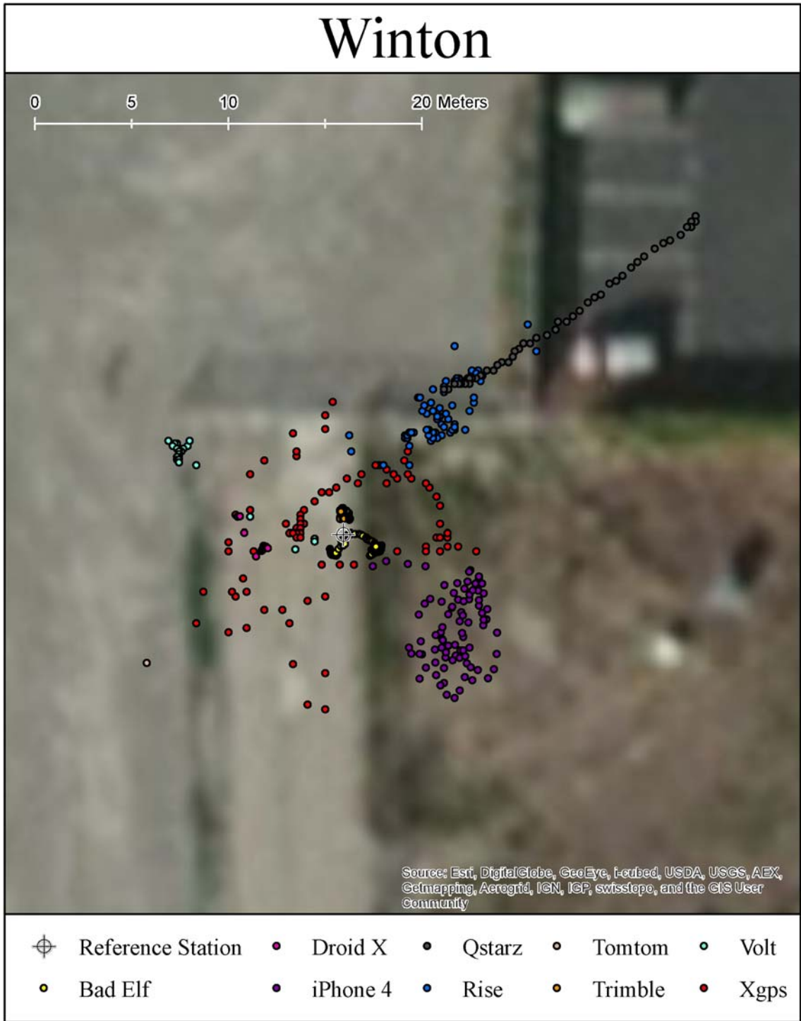
Figure 5. Data point distribution at the Winton CORS site
