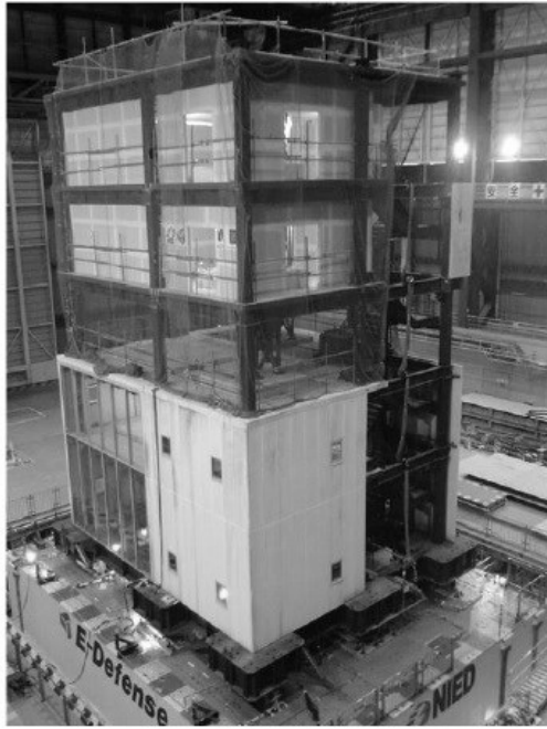
Figure 3.7. Structure Positioned on Shake Table at E-Defense (Ryan, n.d.)
