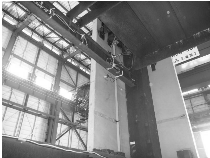
Figure 4.4. Accelerometer Instrumentation on Inside Face of Panel (Photo credit: Maggie Ortiz, 2011)
