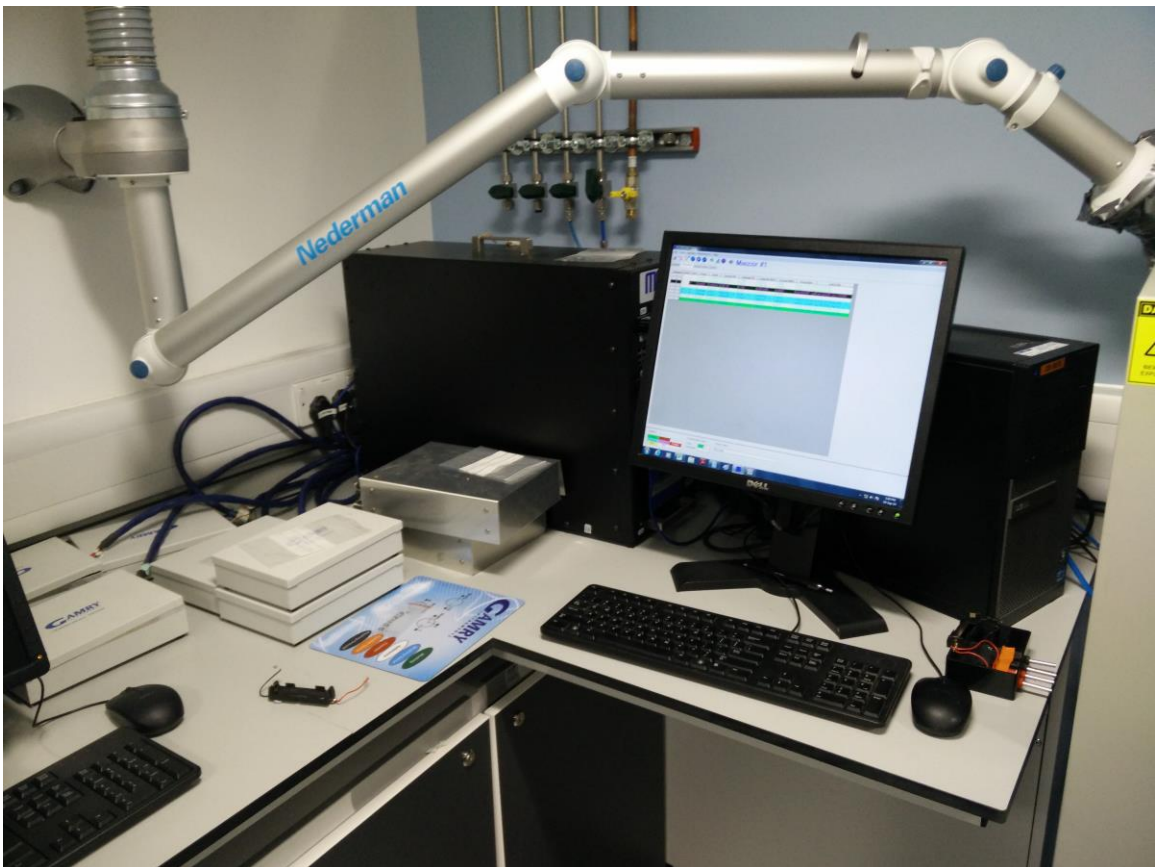
Figure 16. Photo of the Maccor charge cycling apparatus, connected to a PC for control and measurement.
