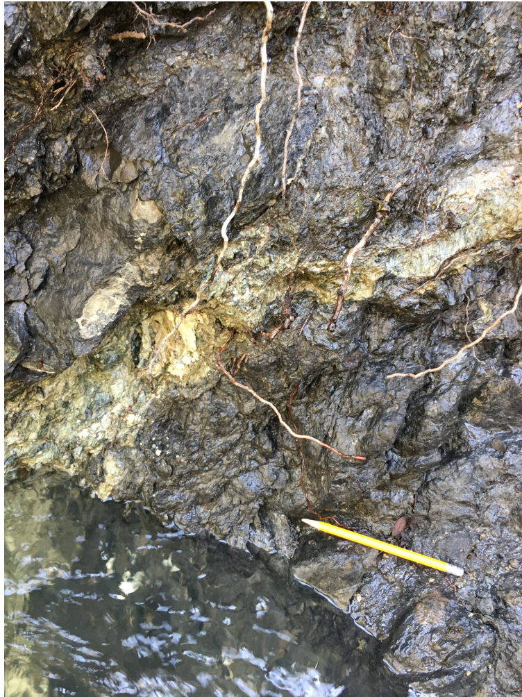
Figure 11: Sheared meta-greywacke within the fault gouge at Site #3. Note the light green tremolite vein cutting along the fault plane.
