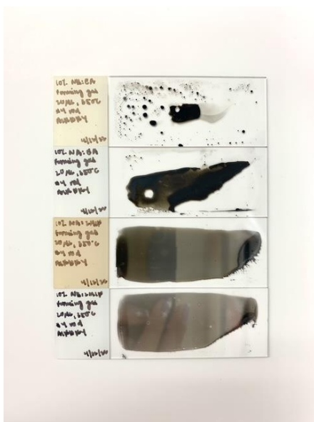
Figure 2. Nickel films made with nickel inks Mayer deposited onto uncoated glass slides and heated to 350 \text{ }^\circ\text{C} in a purged tube furnace under vacuum with flowing forming gas ( 5\% \text{ H}_2 in \text{N}_2 , 0.5 \text{ L}/\text{min} ). From top to bottom: 10\% \text{ w}/\text{w} nickel (II) butyrate in ethanolamine, 10\% \text{ w}/\text{w} nickel (II) acetate in ethanolamine, 10\% \text{ w}/\text{w} nickel (II) acetate in dimethylethanolamine, 10\% \text{ w}/\text{w} nickel (II) butyrate in dimethylethanolamine.
