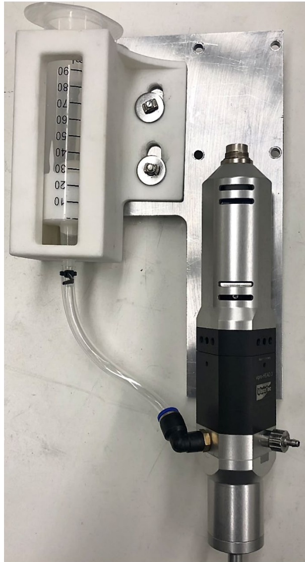
Fig. 2. Physical extrusion subsystem assembly not including the top cover of the feedstock holding bracket introducing compressed air.
