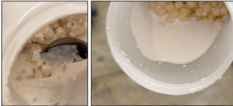
Fig. 7. Visual difference between 60 vol% solids loading (left) and 55 vol% solids loading (right) without using binder.
