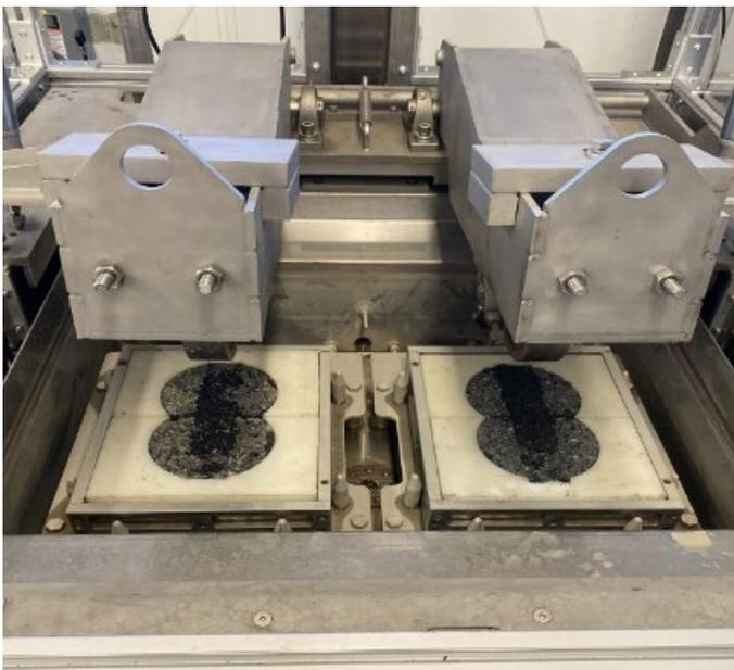
Figure 2. HWT Samples During Testing
