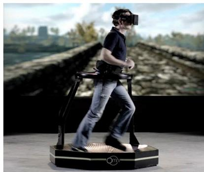
Example of omnidirectional treadmill combined with VR
